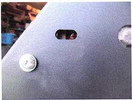
The sideshaft sprocket now also has a window so that the timing belt position can be checked at any time without having to remove the cover.
