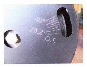
The same values can now also be at the top of the camshaft. It is helpful to colour-code the small hole in the camshaft sprocket with an ink pen.
