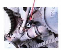
Above the oil filter, screw in the new 70 mm long stud bolt with 2 toothed lock washers and the 8 x 30 screw.
