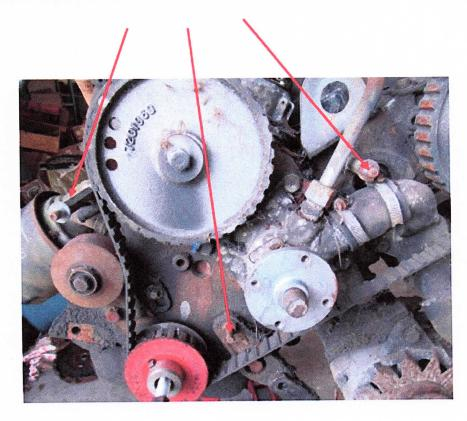
Above the water pump, screw in the new stud bolt with a length of 52 mm with toothed lock washers.
