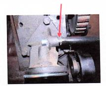
Above the crankshaft, screw in the new stud bolt with a length of 31.5 mm with toothed lock washer.
