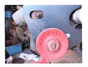
On the crankshaft pulley you can now also see how far the ignition runs at medium speed in the early direction. If everything is working properly, this should be at least 35 degrees at approx. 2500 rpm, if not, correct the vacuum adjustment or the centrifugal force adjustment in the distributor.
