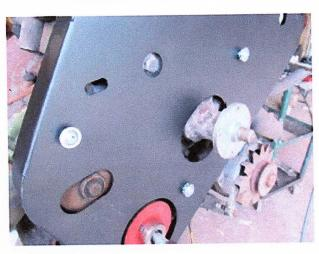
Tighten all stud bolts firmly with the water pump pliers. Now put on the new cover and screw it on with the pan-head screws and toothed lock washers.
