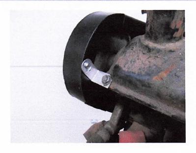
Screw the sheet metal angle on the back with the M 5 screw and the washer.
